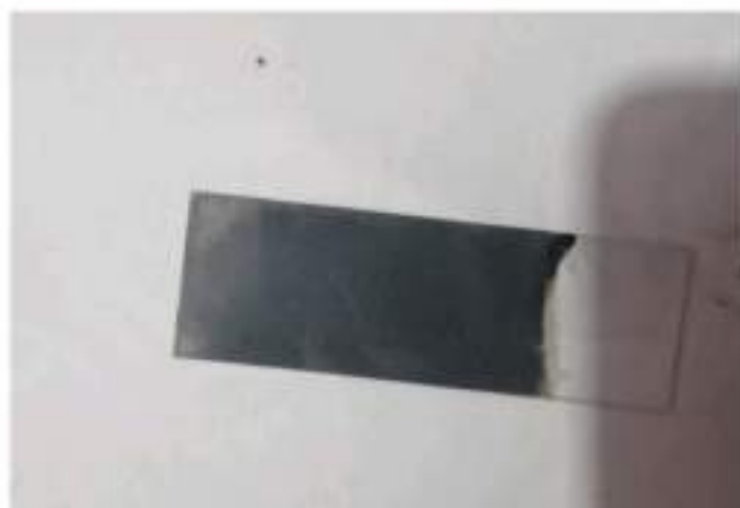
Fig4.2.1: lead Sulphide (PbS) thin film by chemical bath deposition
