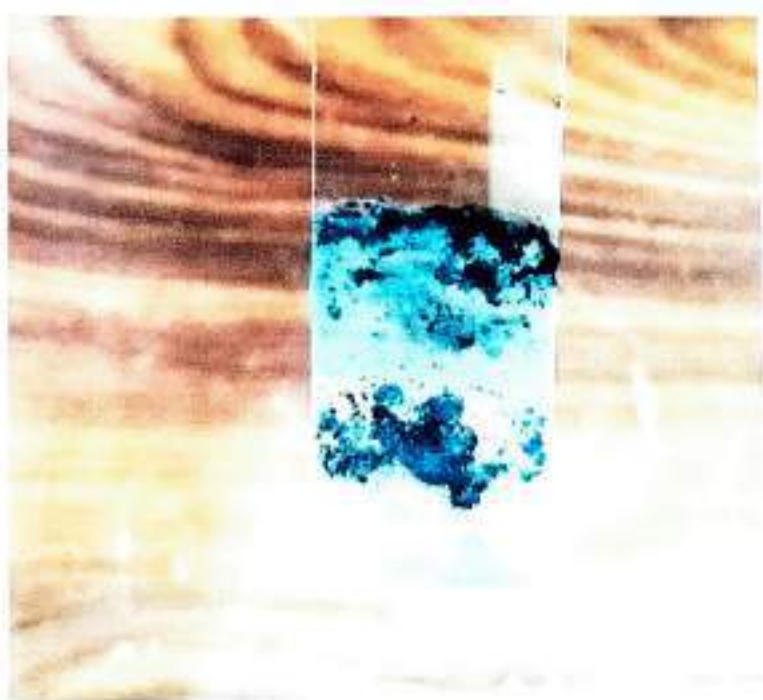
Fig.8 : Lead Selenide (PbSe) thin film by chemical bath deposition
